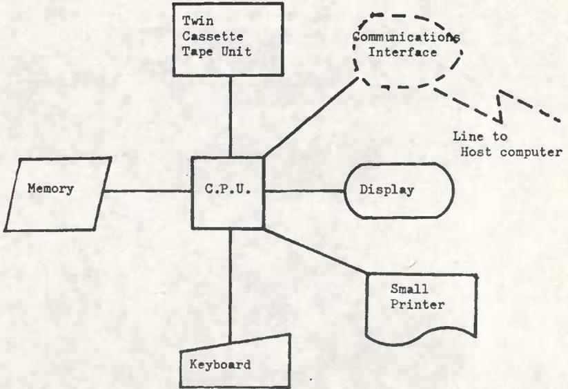
Figure I Elements of an intelligent terminal. The dotted part - access on-line to a larger computer - is not essential.
