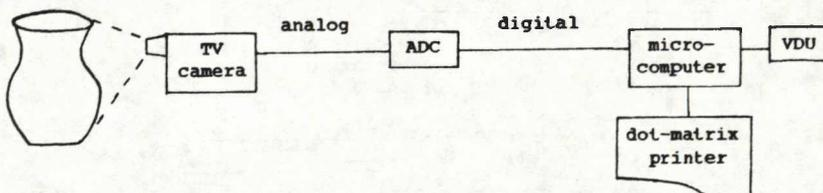
Figure 3: Picture capture by a TV camera and microcomputer.
