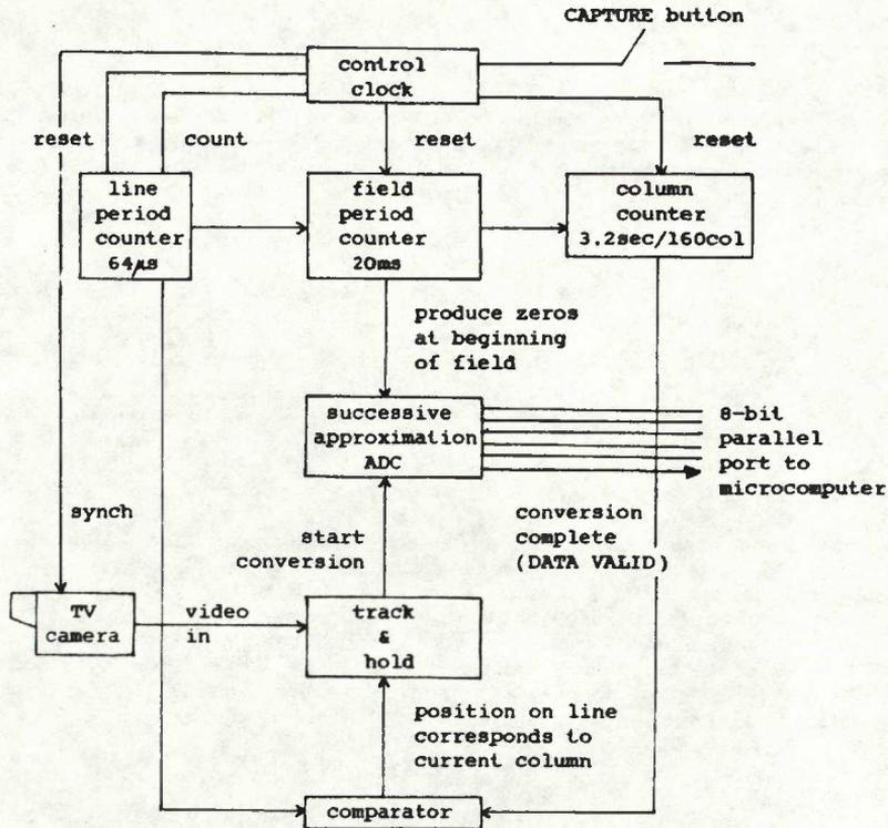
Figure 2: Simplified circuit diagram for the interface
