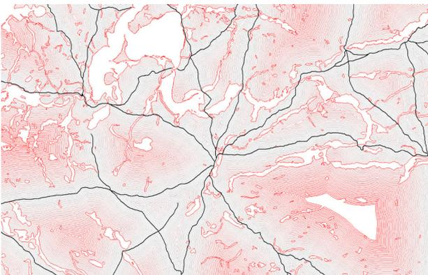
Fig. 7. Buffer-analysis of the highway-network. The distance between buffers is 200 meters. Sea, lakes and larger wetlands are subtracted.
