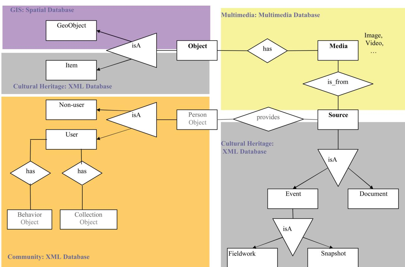
Fig. 6. Three kinds of database technologies are applied: spatial database, XML database and multimedia database.
