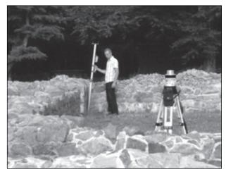
Figure 4. Using the 2-metre long "javelin" probe to survey wall foundations of PC1 (see Fig.7) (iSpace transmitter in foreground).
