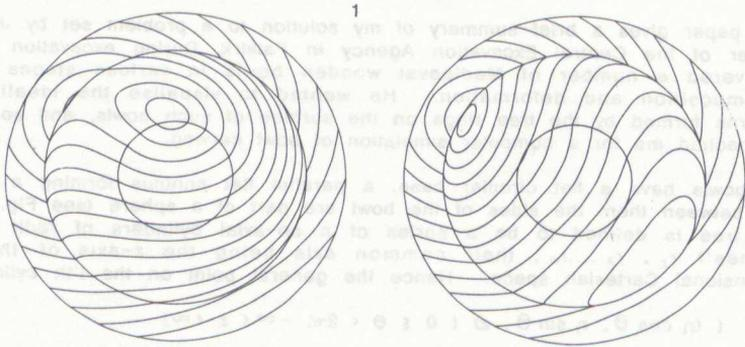
Fig. 1 shows the bowl cut from a tree with rings of radii 0.5, 1.0, 1.5, ...., where  $\underline{c} = (2, 2, 2)$ ,  $\underline{p} = (1, 2, 0.5)$ ,  $f_1 = 0.1$ ,  $f_2 = 0.9$  and  $f_3 = 1.3$ .
