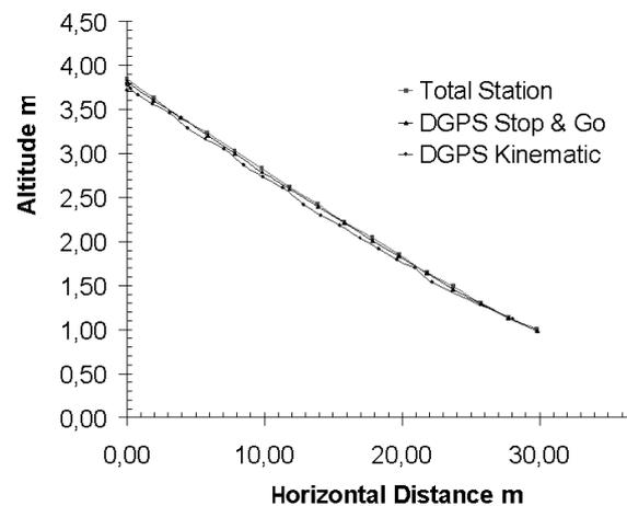
Figure 3: The graph shows the degree of shifting of the Z coordinate according to the method used for the acquisition. The values are included in the expected trend of 2-3 cm.
