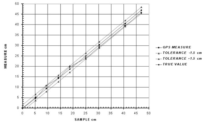
Figure 2: The graph shows the instrument's variable vertical range. The measured value falls into the instrument's tolerance range according to that declared by the producer.
