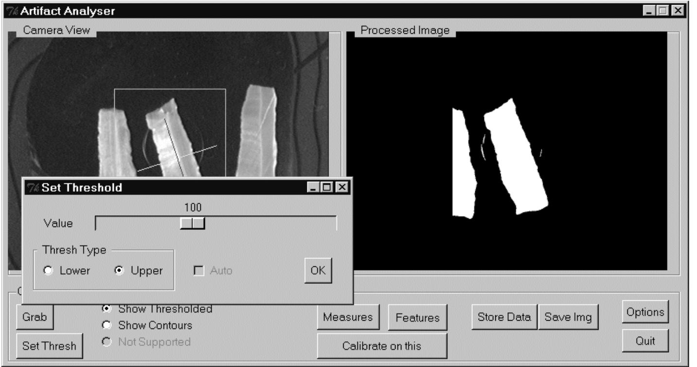
Figure 3: Image of the interface, showing the processing of the thresholding function.
