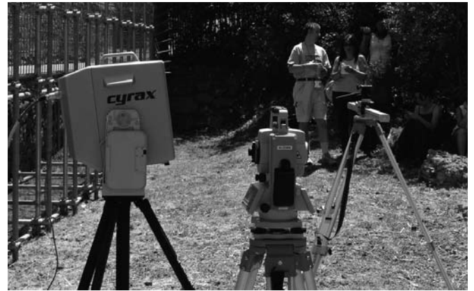
Fig. 11. Integrated acquisition by laser scanner, total laser station and camera for stereo photography.
