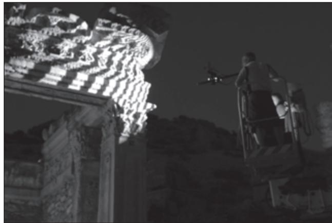
Figure 2. 3D Scanning with structured light scanner at night.
