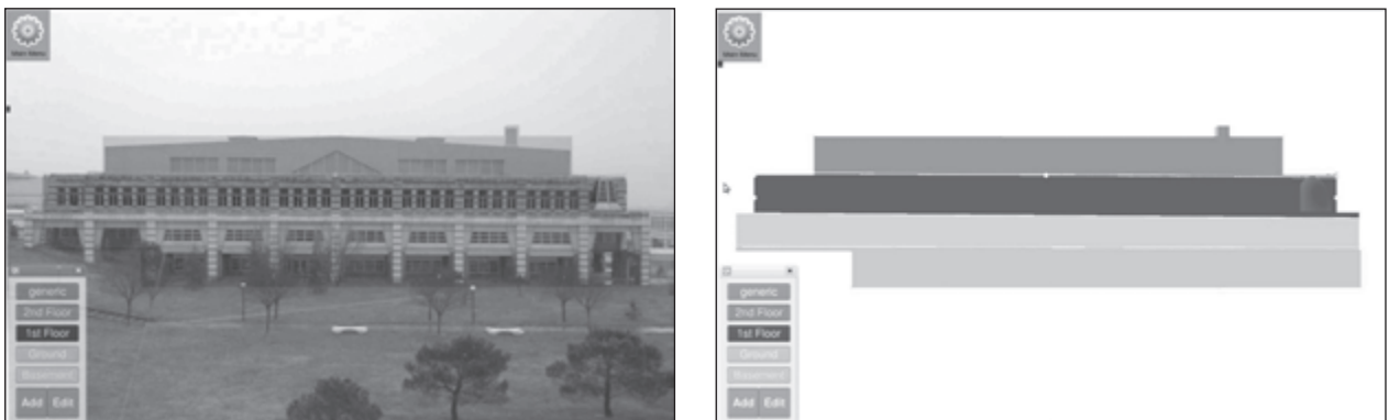
Figure 8. After generating volumetric regions as spatial components, four different annotations are created. These are, from top to down; 2nd floor, 1st floor, ground floor and basement.
